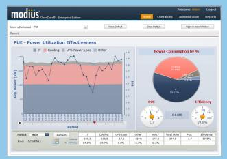
After implementing the energy-saving measures, the company's data center managers used OpenData's real-time data collection and analytic capabilities to confirm the accuracy of the savings estimates provided by the local utility. Comparing measurements taken in the original assessment with results after implementation of the projects, the company found that the projects yielded the expected energy savings.
